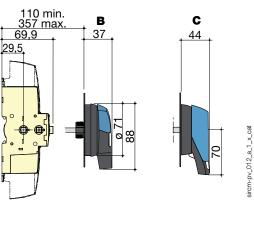
A. 4 poles B. S0 type handle C. S1 type handle 1. Maximum 2 "M" type auxiliary contact modules 2. Maximum 2 "U" type auxiliary contacts
