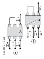
A. Front switch. B. Rear switch. 1. Circuit 1 2. Circuit 2
